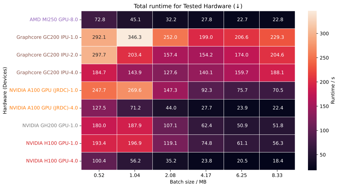
Figure 50: AP5 Time: Time-to-Solution on different hardware as a function of batch size. ap3-runtime-vs-hardware-heatmap
